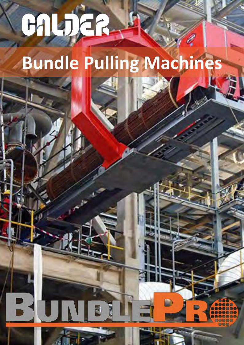
The safe and efficient method of extracting tube bundles. From 5 tonnes to 100 tonnes, we have the machine to make your job easier. Twelve models of aerial bundle extractor along with truck-mounted and self-propelled machines offer you the solution to the majority of tube bundle handling jobs.
